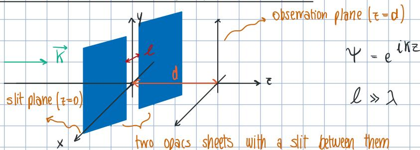
We can use the scalar theory of diffraction (derived from the Huygens principle) to measure the intensity of the field at a certain distance  $d$ .
