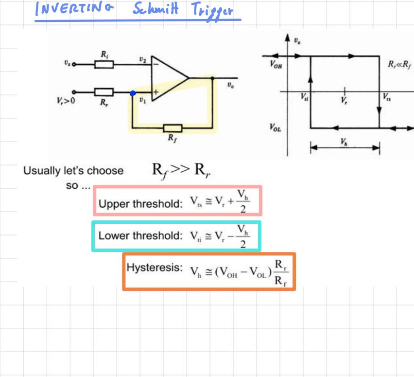
To introduce the hysteresis in a comparator stage, it is sufficient to add slightly positive feedback to the OpAmp through the resistors  $R_f$  and  $R_r$ , as shown in Fig. 2.50. The signal  $v_s$  is applied to the non-inverting input terminal through the  $R_i$  resistance (irrelevant to the operation of the system) while the external reference voltage  $V_r$  is applied to the resistance  $R_r$ . The voltage
