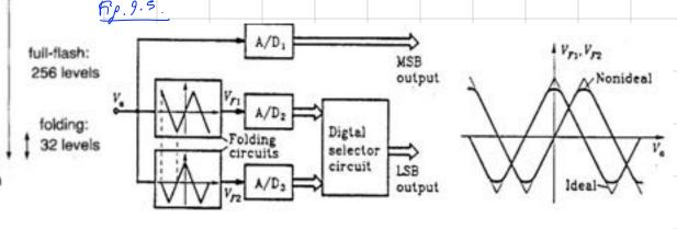
uple of a double folding circuit, in order to avoid non idealities of folded edges . other folding shapes can be used ..
