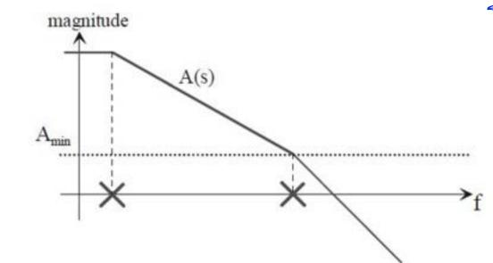
Fig. 3.73: A<sub>min</sub> represents the minimum gain that can be used without needing any compensation.
