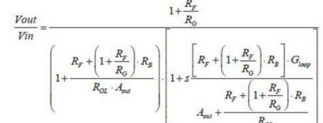
maximize R<sub>OL</sub>·C<sub>COMP</sub> and show how R<sub>OL</sub> will be made through the collector resistor (very high resistance).
