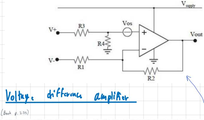
A simple solution to the problem arising from the need that has just been mentioned might be the so-called Differential Amplifier depicted in Figure 3.1. In this configuration, many non-idealities impair the Common Mode Rejection, and the high common mode gain is the heaviest limit of the Differential Amplifier. In order to have an infinite CMRR, the following two conditions must be met:
