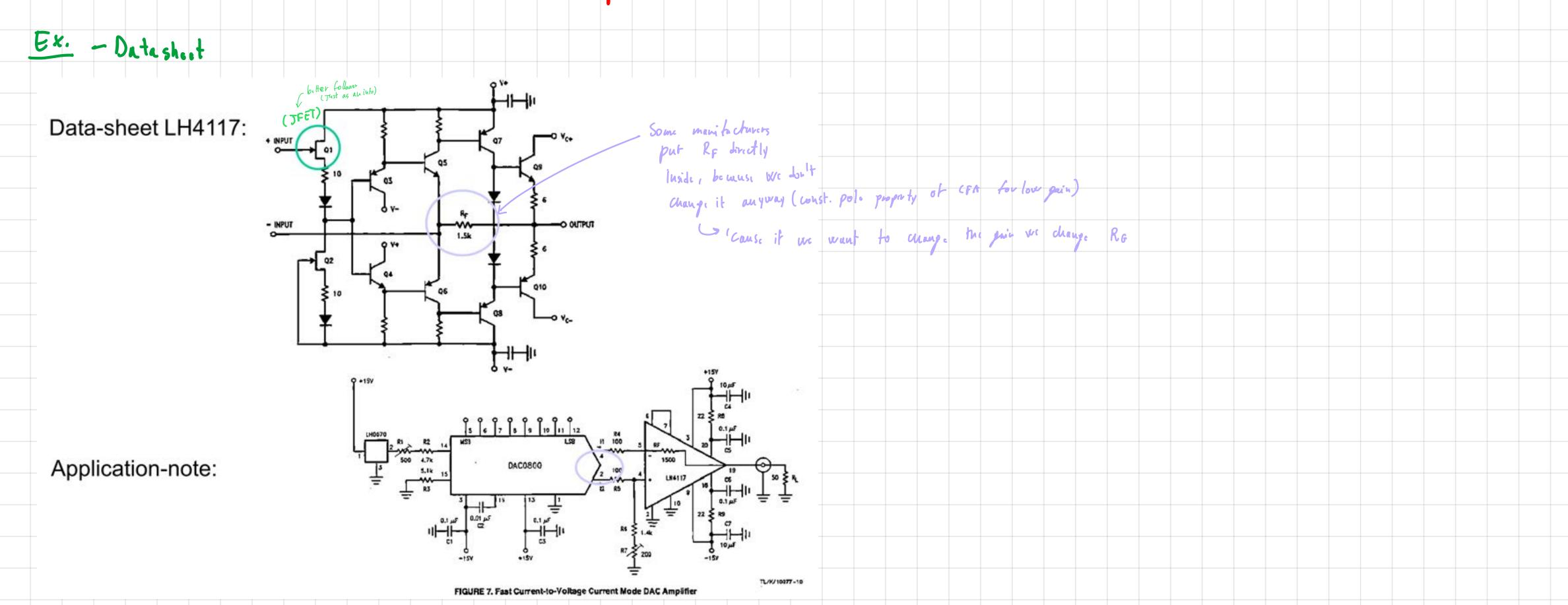
$i_{out} = G_m(I_{control}) \cdot v_{diff} = \frac{I_{control}}{kT/q} \cdot v_{diff} = \frac{I_{control}}{25mV} \cdot v_{diff}$
