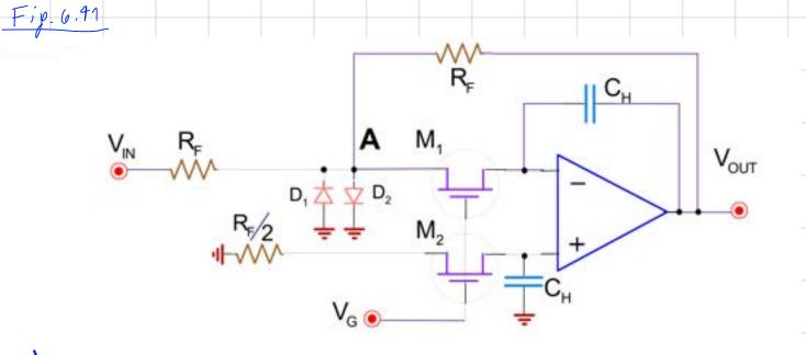
V<sub>G</sub> can have simple low-voltage CMOS levels (0-3.3V), independent of V<sub>IN</sub> the Aperture-Induced non-linearity can be drastically reduced
