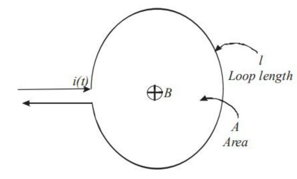
Figure 11. Current loop for the calculation of inductance
