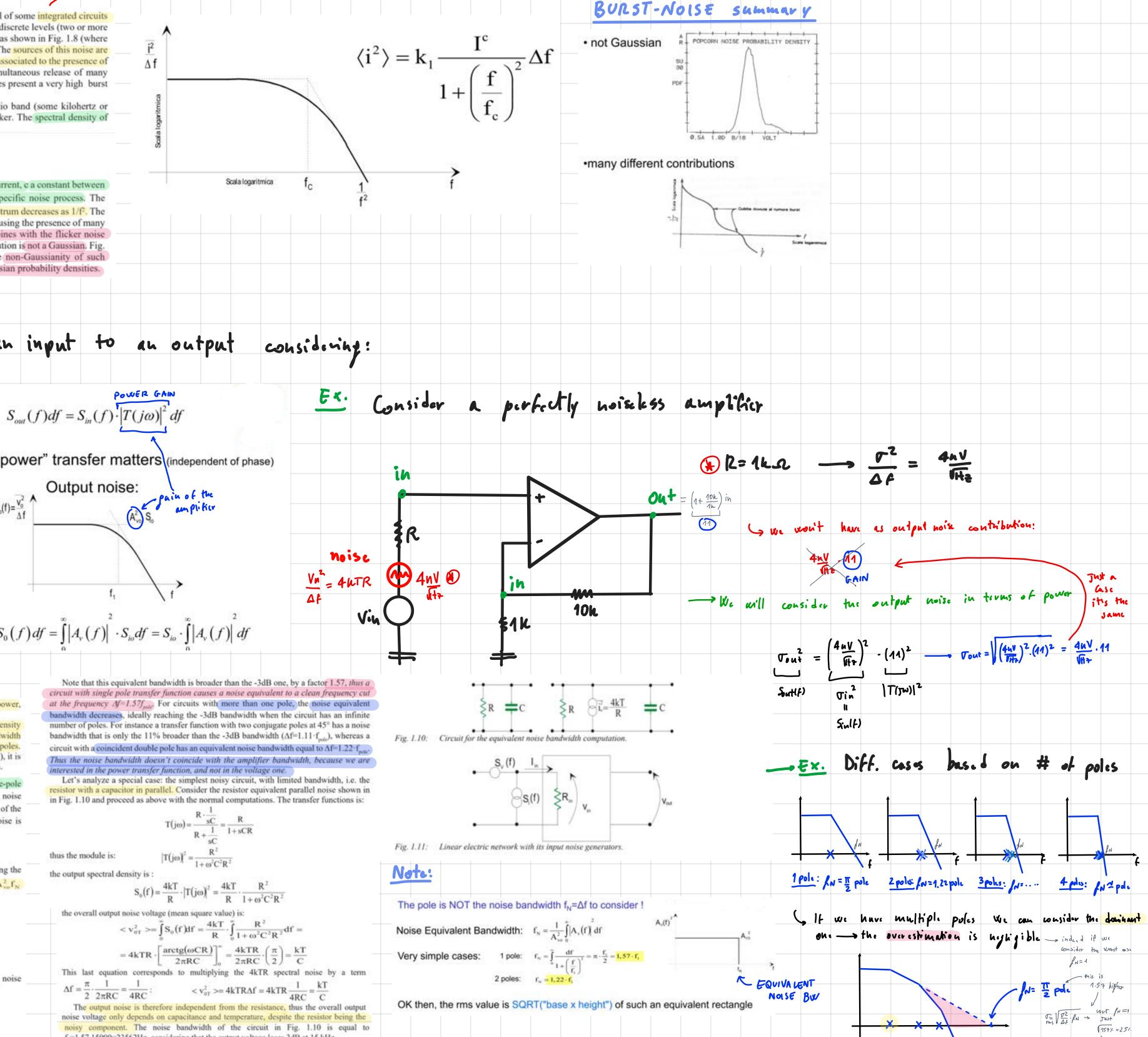
Identical Bode diagram, but for noise only "power" transfer matters (independent of phase)
