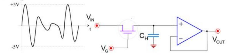
It is obvious that this is a very restrictive condition, much more restrictive than the theoretical limit imposed by the Sampling Theorem of  $f_{max} < \frac{1}{2} f_S = (2 \cdot T_{conv})^{-1} = 50 \text{ kHz}.$
