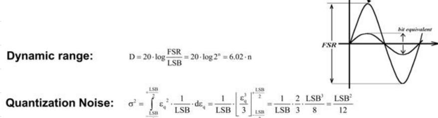
**Ideal S**ignal-to-**N**oise **R**atio:  $SNR|_{max} = \frac{\max \text{ signal power}}{\min \text{ noise, just quantization error}} = 10 \cdot \log \frac{(FSR/2\sqrt{2})^2}{(LSB^2/12)} = 6.02 \cdot n + 1.76$
