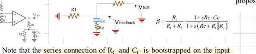
signal since the stage reads the voltage on the positive terminal and gives it back the same (at least in the case of an ideal OpAmp) to the inverting one. Then, there will be no current flow in the series connection. Since this network does not affect the real gain, but only the gain  $\beta$ , it will allow compensating the stage without changing its closed-loop gain.
