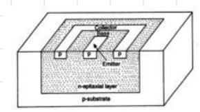
Fig. 1.17 A pap lateral transistor
