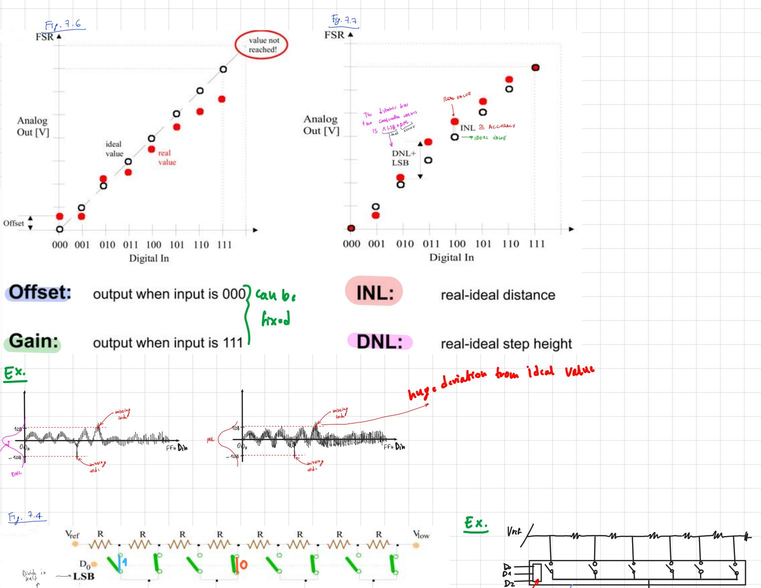
This circuit offers the advantage of ensuring an intrinsic monotonicity of the conversion and of needing identical resistance values, which is easily achievable with high accuracy.
