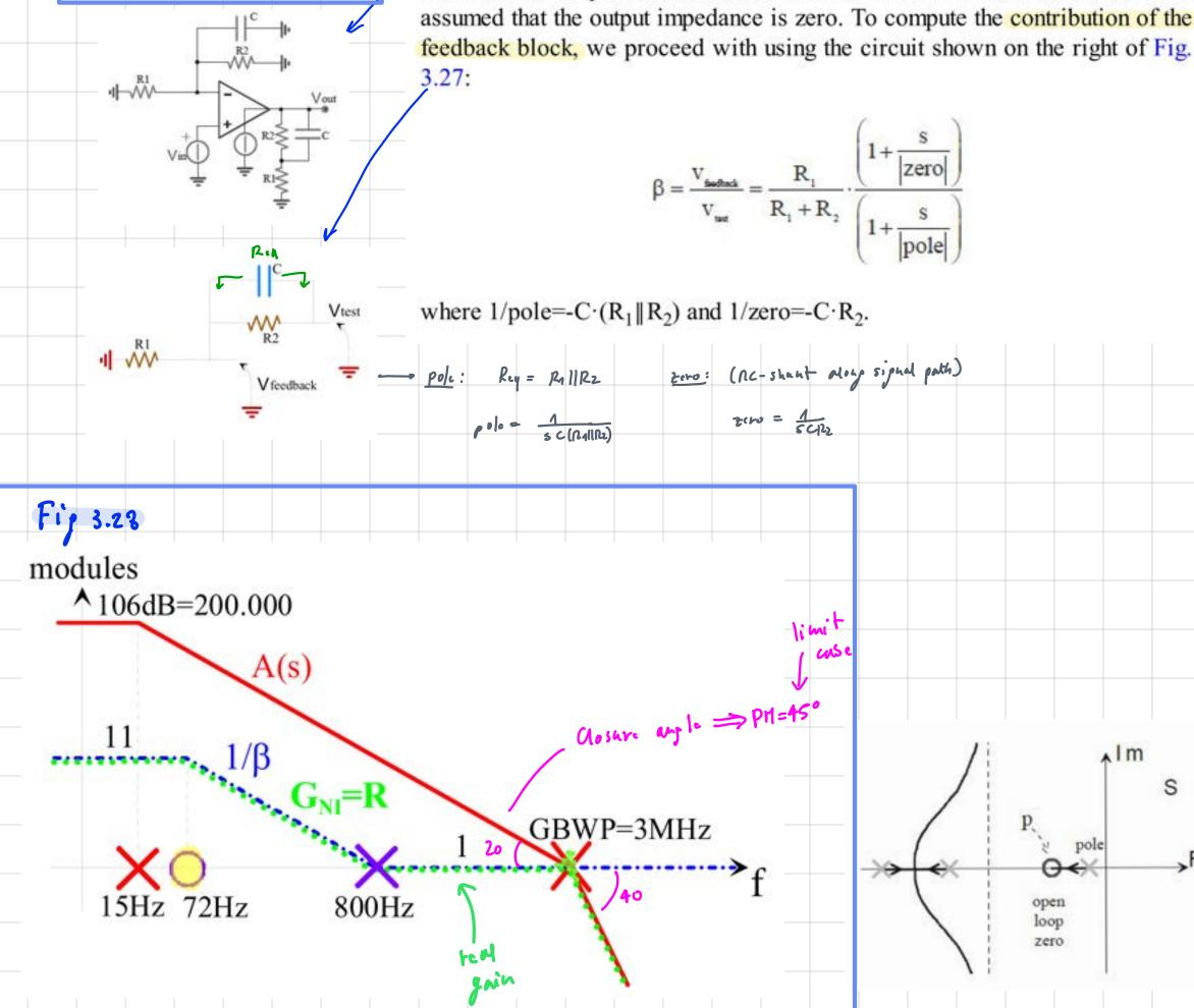
which is 11 at frequencies below the pole (of  $1/\beta$ , which is the zero of  $\beta$ , which is  $1/C \cdot R_2 = 72$ Hz) and 1 at frequencies above the zero (when C becomes a short circuit with respect to  $R_2$  and the stage gets buffer connected).
