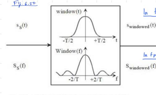
Fig. 6.27: Windowing effect on original sequence samples.
