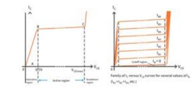
Figure 9: Collector characteristic curves
