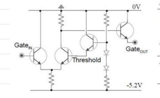
Fig. 6.33: Example of a differential stage for the sampling command.
