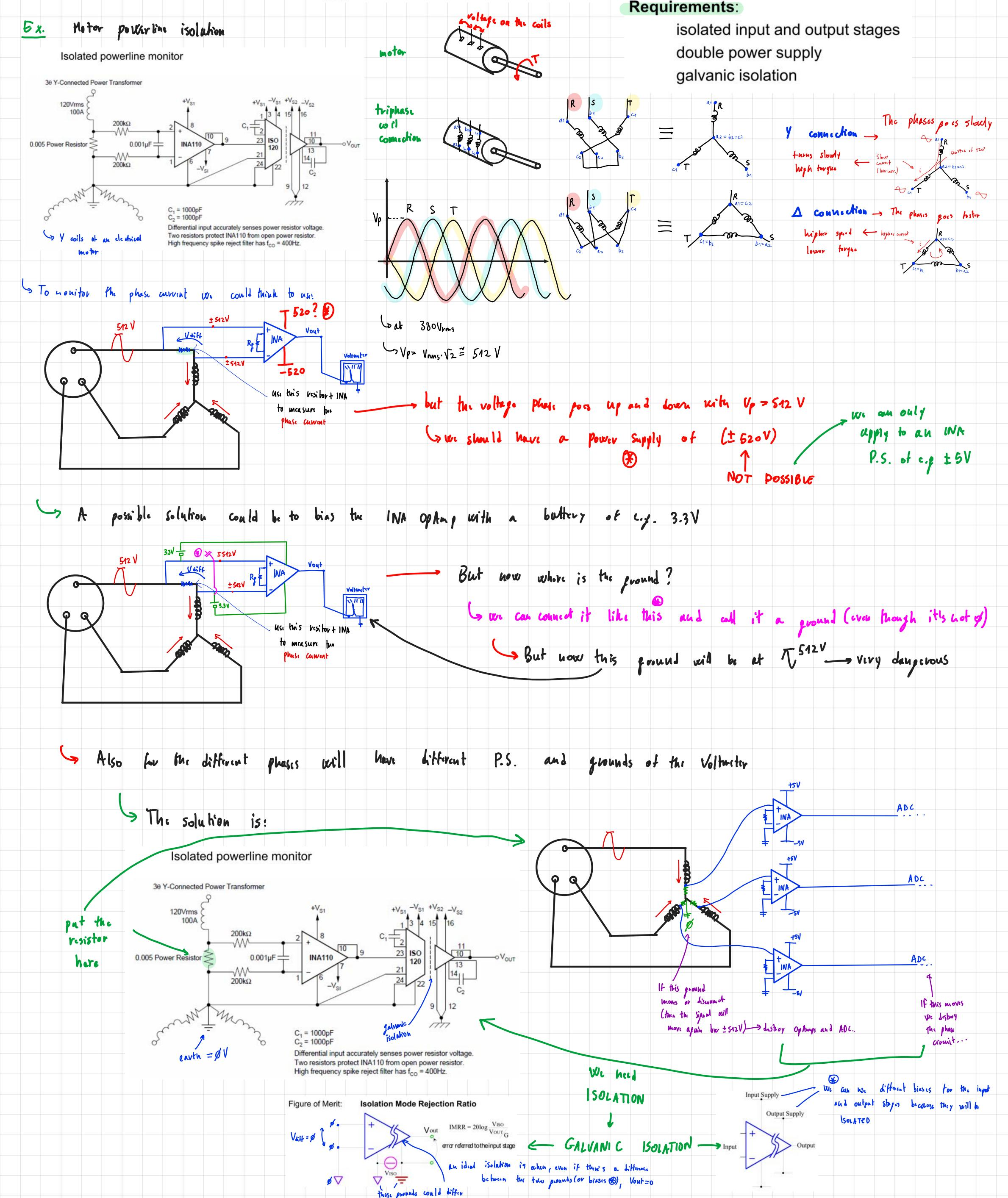
The IMRR does not suffice to satisfactorily indicate the capability of the ISO to isolate the two worlds. Particularly, the *steep edges* can overload the amplifier, causing non-linearity, offset errors, and saturation effects. To have a response on the behavior of the ISO from this point of view, we can use the TRANSIENT IMMUNITY (TI) expressed in  $[V/\mu s]$ . For example, for the ISO122, we have:
