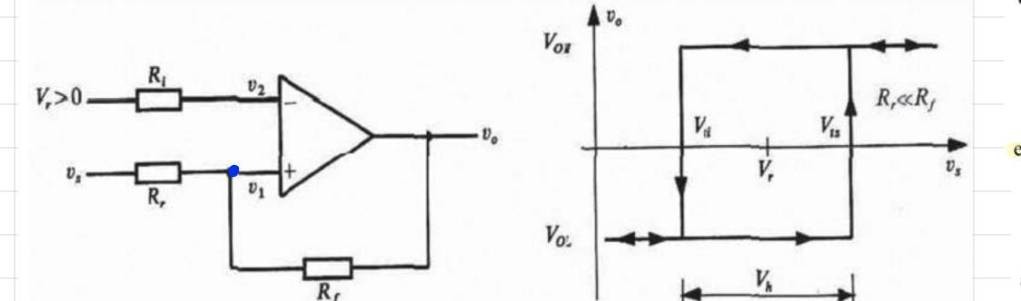
The non-inverting Schmitt Trigger is similar to the inverting configuration, but the input signal  $v_s$  and the reference  $V_r$  are reversed, as shown in Fig. 2.51. With an analogous reasoning, as for the inverting configuration, we have:
