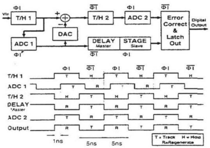
Fig. 9.20: Pipelined ADC timing graph.
