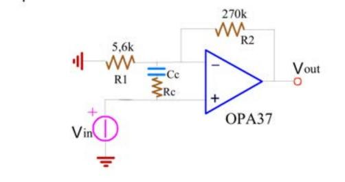
R<sub>c</sub> C<sub>c</sub> are bootstrapped on the input signal, hence they have no role in the circuit (what's up here then?!?!)
