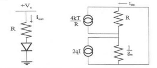
Fig. 1.19: Computation of the current noise in a biased junction (left) and an equivalent circuit for small signals (right) with the noise generators.
