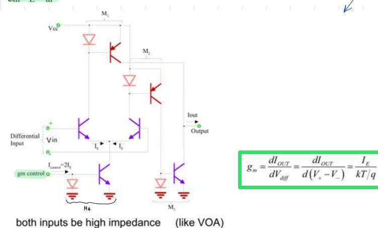
both inputs be high impedance output be current transconductance gain
