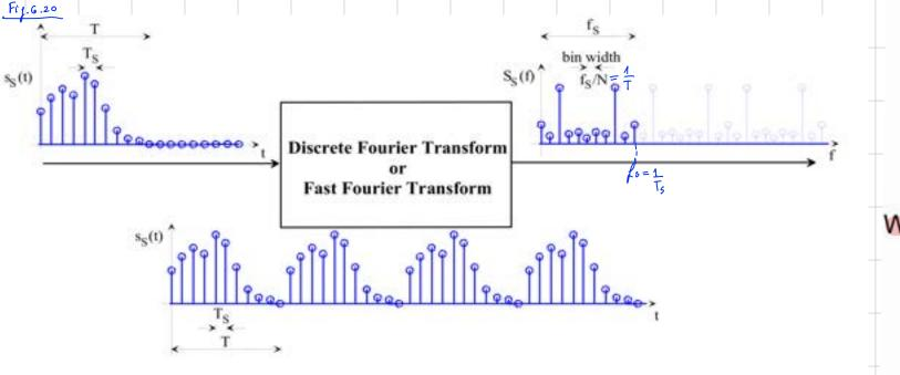
The FFT algorithm trusts on the periodicity of the input sequence
