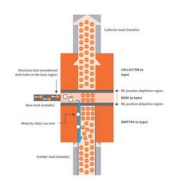
Figure 4: BJT operation showing electron flow
