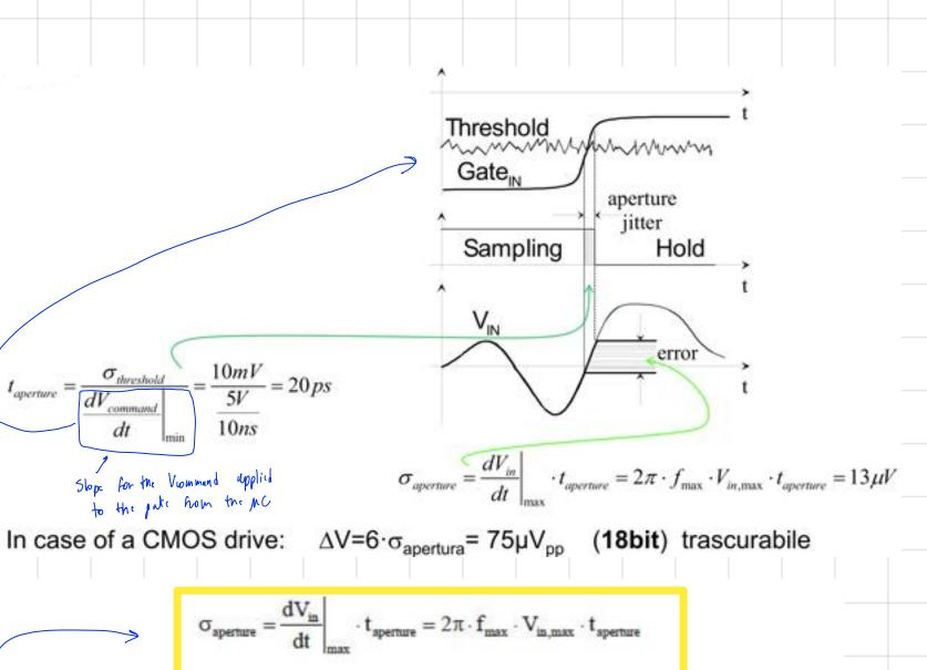
In this project, we have an *rms* value of  $\sigma_{aperture}=0.628\mu V$ , corresponding to a statistical error with a ranging of about 3.8µV peak-to-peak, which is nonnegligible in this case.
