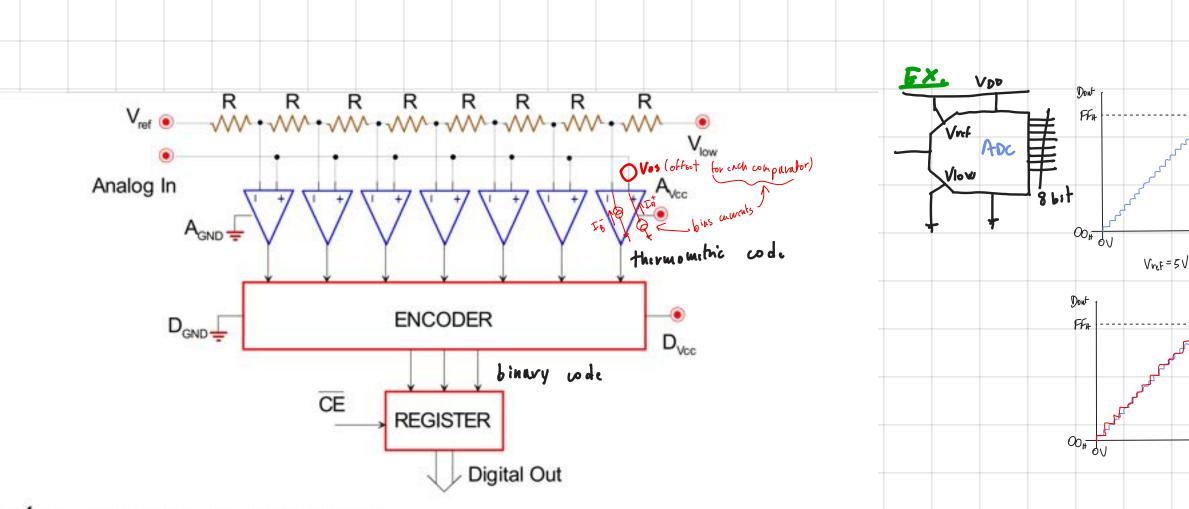
Components: 2<sup>n</sup> resistors and 2<sup>n</sup> comparators
