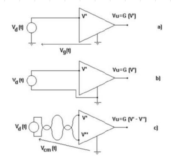
Fig. 1.5: Connection schemes of a sensor to an amplifier: a) single-ended through ground; b) single ended through two wires; b) differential sensing.
