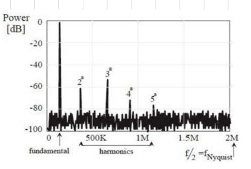
Fig. 7.12: Spectrum of the output signal of the DAC: we can see the sine wave of interest, the spurious harmonics, and the background noise; each histogram has a width that is called bin width.
