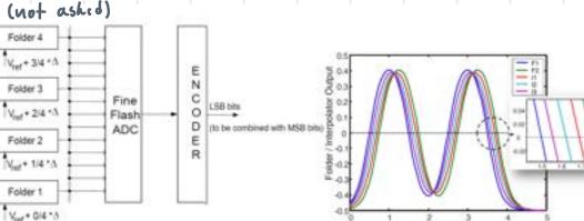
Example of 4 folders with 4 folds each, so 16 zero-crossings, hence + 4 LSB bits ... anywat upper limit... due to added complexity.
